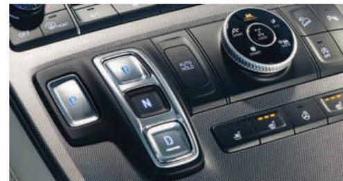
Shift-by-Wire push-button gear selection
