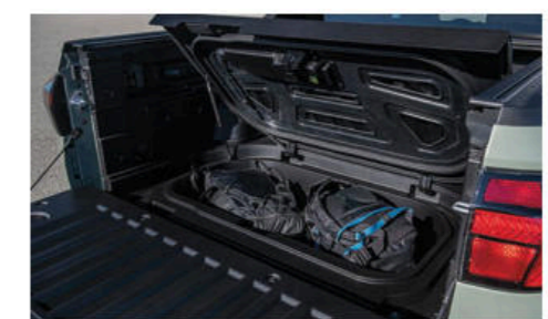
Lockable under-bed storage compartment
