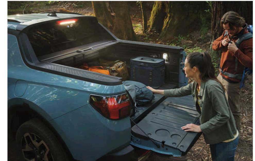
Sheet molded composite bed with rail system, adjustable tie-down cleats and LED bed lighting
