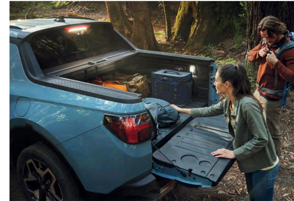
Sheet molded composite bed with rail system, adjustable tie-down cleats and LED bed lighting
