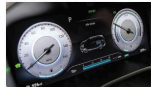
12.3" digital LCD instrument cluster
