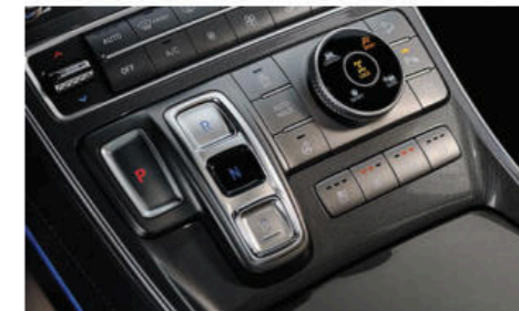
Push-button Shift-by-Wire gear selection
