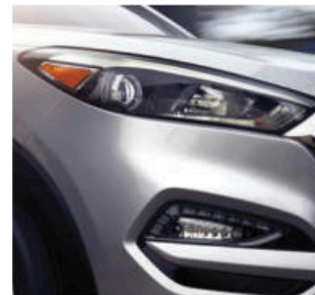
High-Intensity Discharge headlights with Dynamic Bending Light
