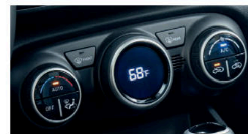
Automatic temperature control
