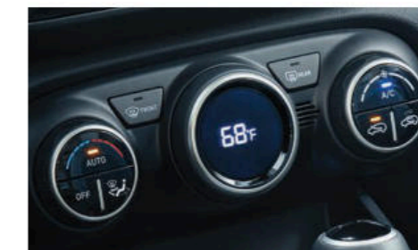
Automatic temperature control
