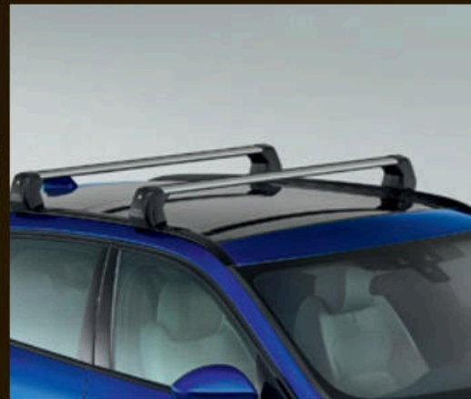
Roof Cross Bars
