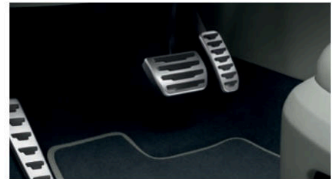
Stainless Steel Sports Pedals VPLHS0044 – Automatic Transmission vehicles Stainless steel pedals feature a bright design and hidden fixings for a clean finish. Stainless Steel Sports Footrest VPLVS0178 Complementing the sports pedals, the footrest is manufactured from stainless steel and features a satin finish.
