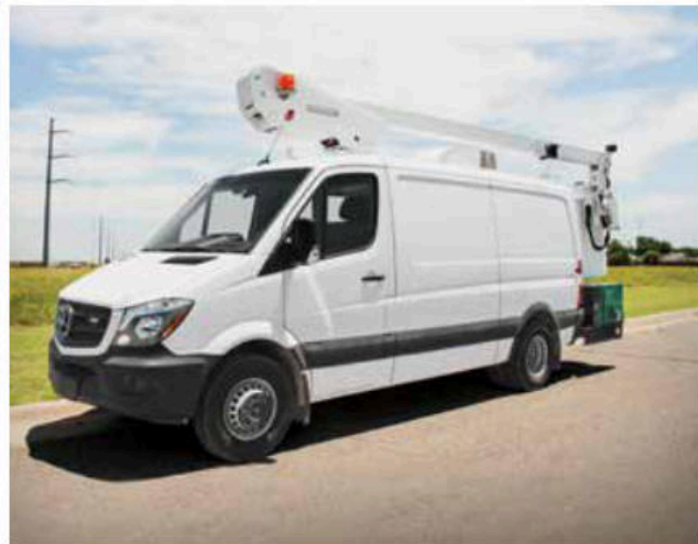
Aerial lift conversion done by Equipment Technology, LLC — A Palfinger Company.
