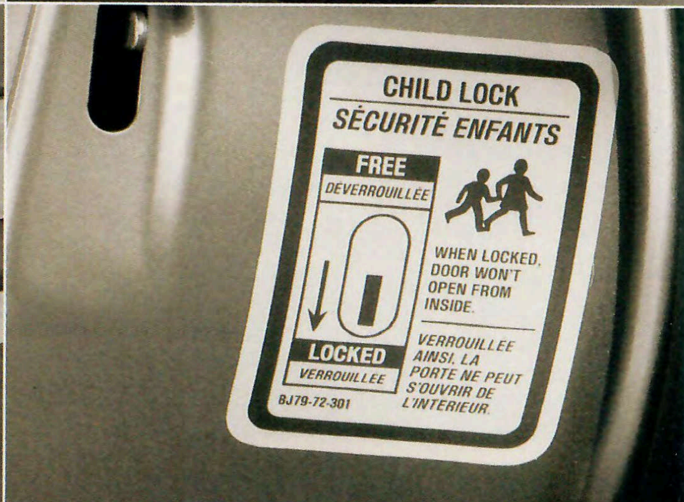
Child-proof door locks in the rear doors of all Mercury sedans as well as Villager keep children in back from accidentally opening the doors from inside the car, while allowing parents to still open doors from the outside.
