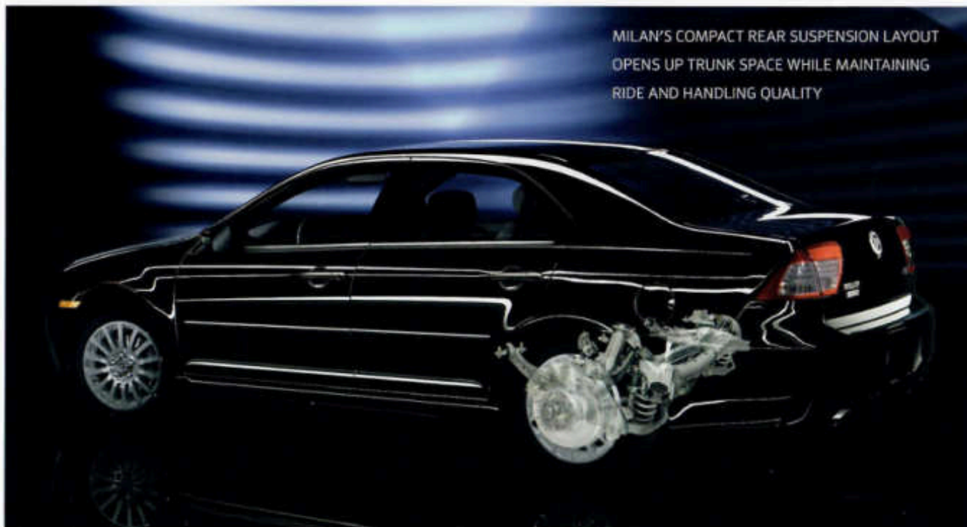
MULTI-LINK INDEPENDENT REAR SUSPENSION
