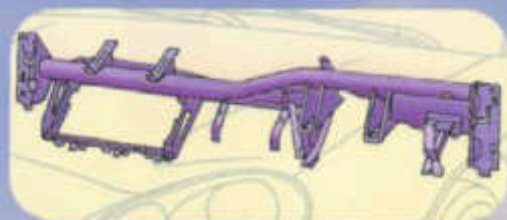
Instrument panel cross-car beam produces a quieter, smoother ride, and better handling.
