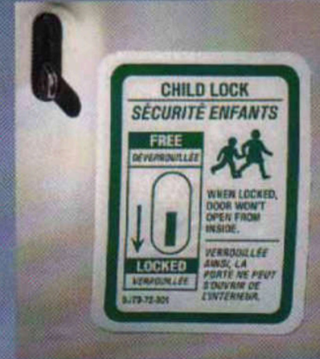
Child-proof rear door locks prevent rear doors from opening from the inside while allowing parents access from the outside.
