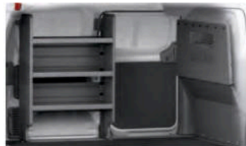
NV200 Compact Cargo 32" shelving unit and a steel or wire partition
