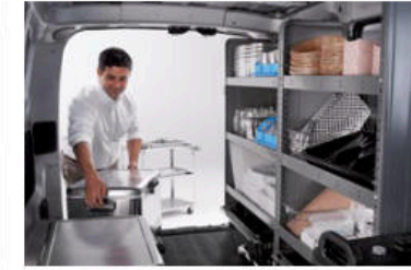
Integrated reinforced cargo-mounting points allow cargo racks, partitions and bins to be securely mounted. 1 Integrated exterior roof rack-mounting points help secure racks. 1
