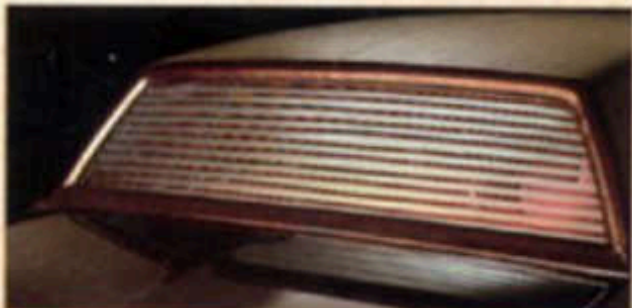
Rear window defogger. Electric filaments in the glass defog the window quickly and silently.
