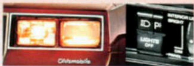
Headlamp-on reminder switch, standard. Sounds and flashes warning when door is opened.
