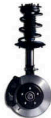
Twin-tube struts with 4-stage valving were engineered exclusively for Intrigue. They provide precise control and quick response.
