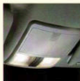
A standard overhead console provides dual reading lamps and storage for sunglasses.
