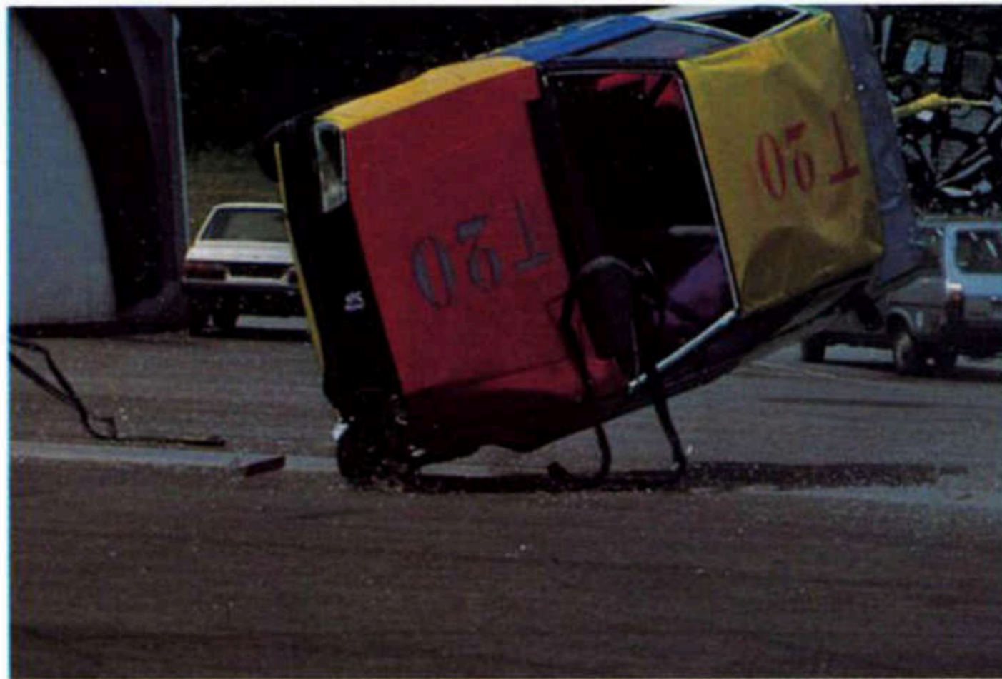
A steel cage protects in the event of a rollover.
