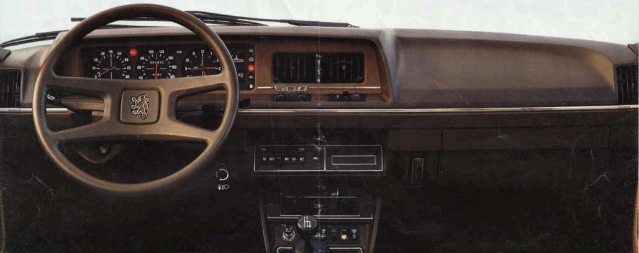
At night, the discrete lighting of the dashboard, coupled with the powerful halogen headlights, ensures perfect visibility of the road without distracting the driver. The beam adjustment control, operated from the inside, allows instant correction of headlight focus when the car is heavily loaded.
