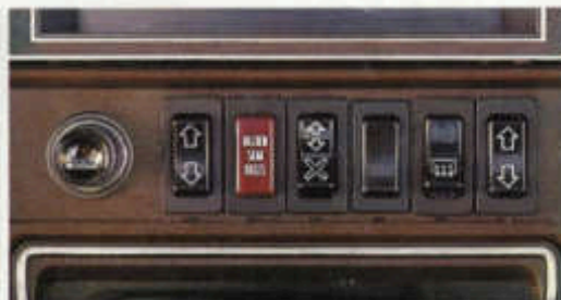
CENTRE CONSOLE , with cigarette lighter and finger tip controls for electrically operated windows.
