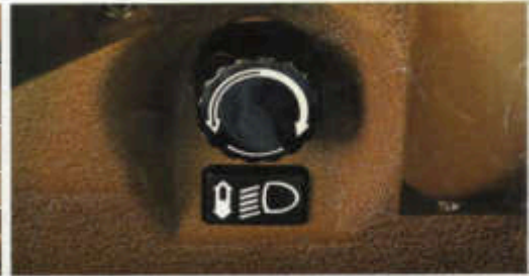
HEADLIGHT BEAM ADJUSTMENT CONTROL , to compensate for heavy loads, operated from the driver's seat.
