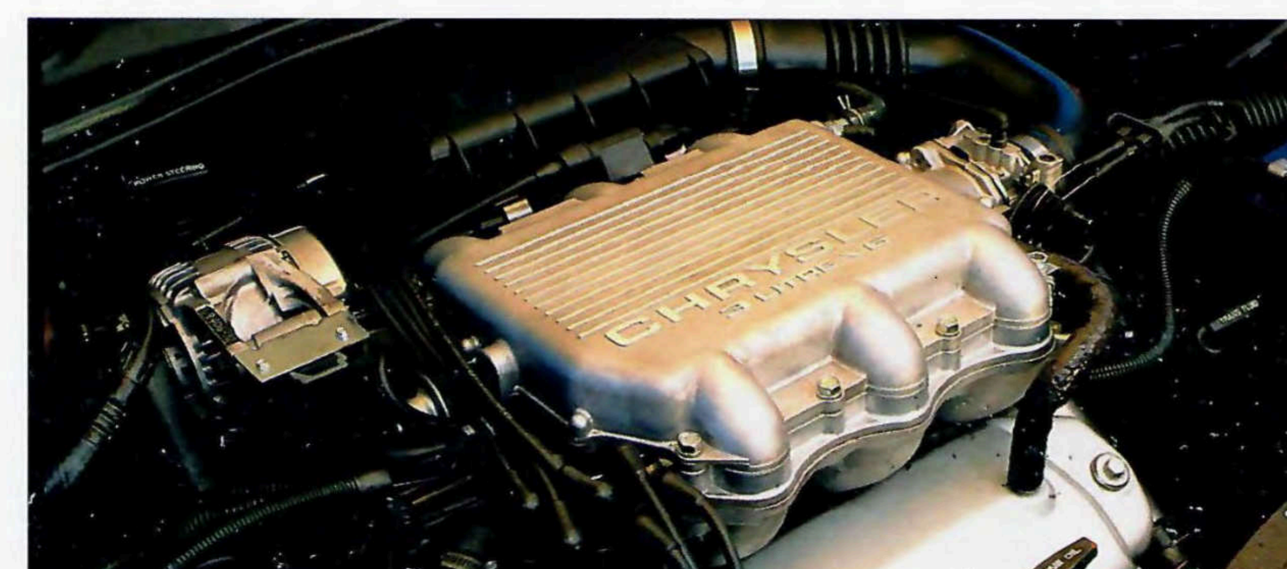
An available 3.0-liter V6 SMPI (sequential multipoint fuel injection) engine is powerful, responsive and quiet running. A lively and efficient 2.5-liter EFI (electronic fuel injection) dual balance-shaft engine is standard on Acclaim. (See page 12 for complete engine details.)
