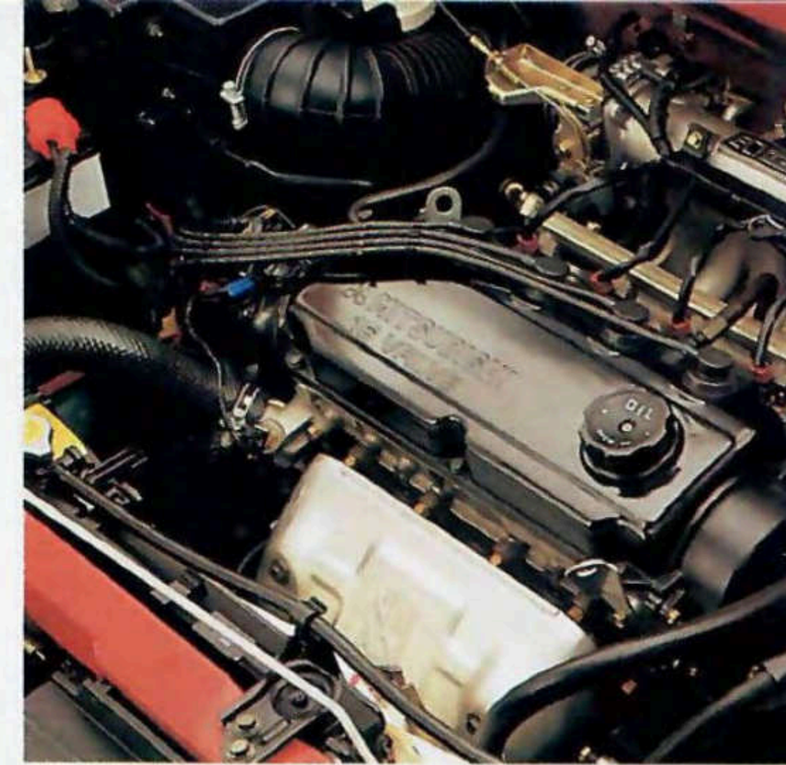
Advanced 1.8-liter 16-valve single overhead cam (SOHC) multipoint fuel injected (MPI) engine is standard.
