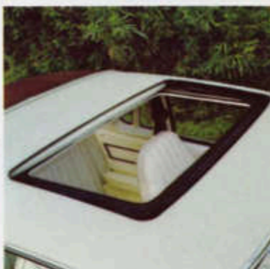
Manually-operated sun roof.
