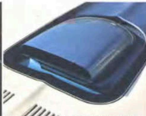
The shaker hood's rear-facing inlet literally "rams" air.
