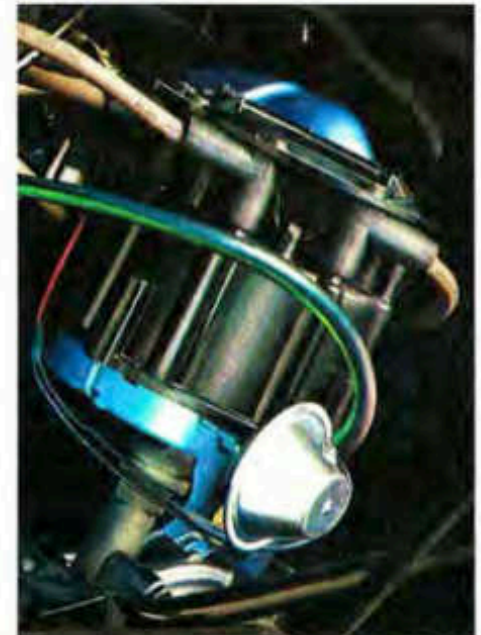
Firebird's High Energy Electronic Ignition zaps up to 35,000 volts of power to the plugs.
