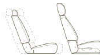
Torrent's "Multi-Flex" sliding rear seat affords eight inches of total travel; slide it forward to maximize cargo room, back for the most rear leg room in the class.*
