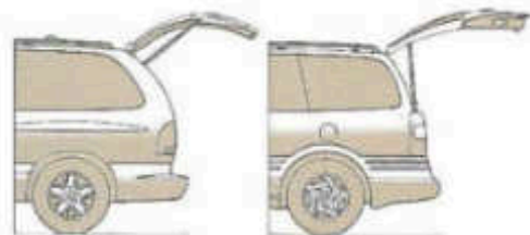
With plenty of head room (compared to loading competitors), Montana's hatch struts (right) are positioned out of the way to further ease loading.
