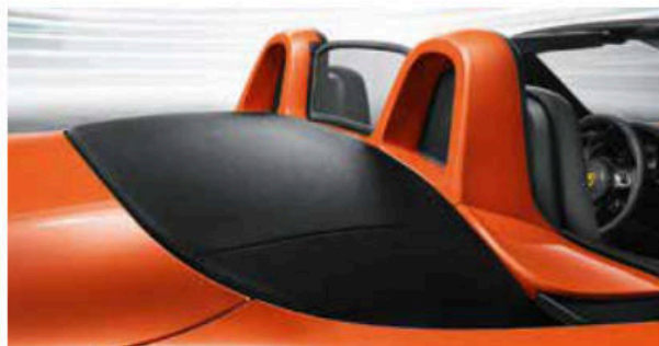
Supplemental safety bars painted in exterior color, net-type wind-deflector grille
