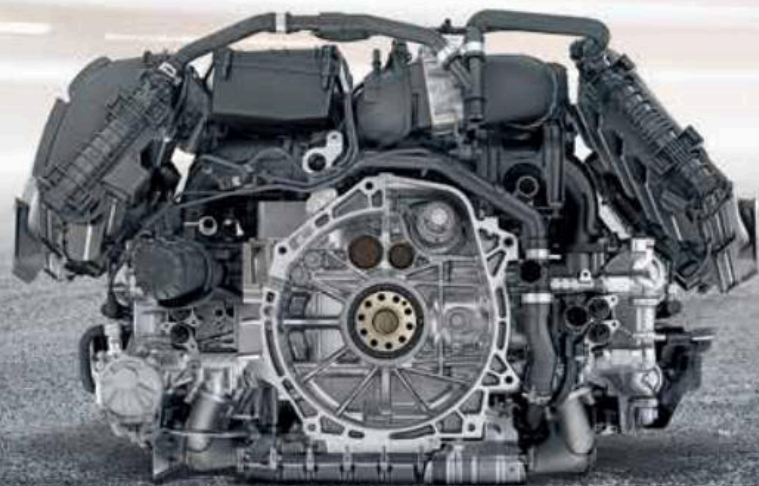
718 Boxster and 718 Cayman: 300 hp at 6500 rpm, 280 lb.-ft. between 1950 and 4500 rpm
