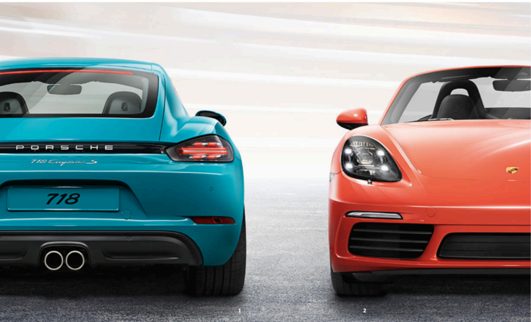
1 LED taillight with four-spot brake light 2 LED main headlight with four-spot daytime running light
