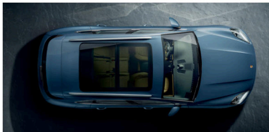
Panoramic roof system
