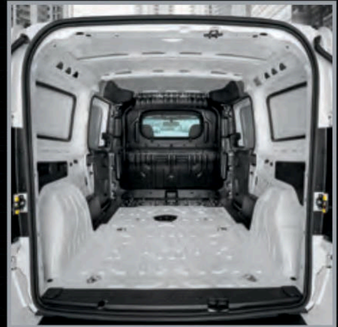
PARTITION WITH WINDOW Available for Tradesman Cargo Van and SLT Cargo Van
