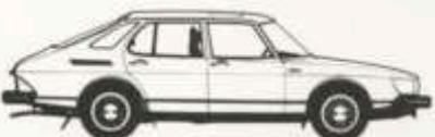
SAAB 900TURBO, FIVE-DOOR. Turbocharged fuel-injection engine developing 135 hp (100 kW) SAE net. Manual gearbox.
