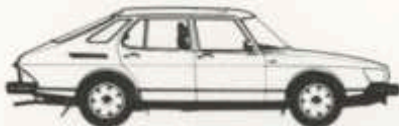
SAAB 900GLE, FIVE-DOOR. Fuel-injection engine developing 115 hp (85 kW) SAE net (110 hp, 81 kW, catalyst equipped). Manual gearbox or automatic transmission.
