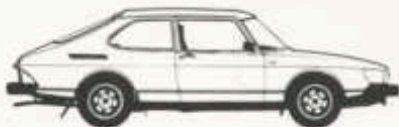
SAAB 900EMS, THREE-DOOR. Fuel-injection engine developing 115 hp (85 kW) SAE net (110 hp, 81 kW, catalyst equipped). Manual gearbox or automatic transmission.
