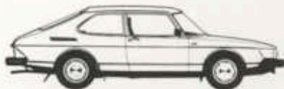
SAAB 900GLI, THREE-DOOR. Fuel-injection engine developing 115 hp (85 kW) SAE net (110 hp, 81 kW, catalyst equipped). Manual gearbox or automatic transmission.
