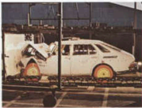
Saab's are designed with front and rear collision zones and a rigid passenger compartment with abundant impact-absorbing material.
