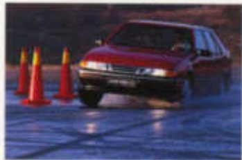
ABS prevents the wheels locking and sliding under braking.
