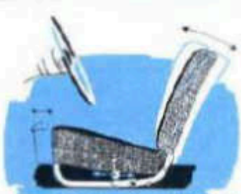
Front seats individually adjustable forward and backward. Adjustable backs, with seven settings.
