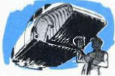
Body-frame unit rust-proofed and undercoated at factory.
