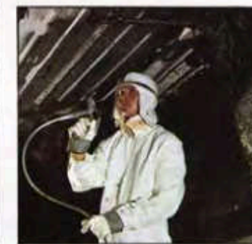
Body undercoated during manufacture.
