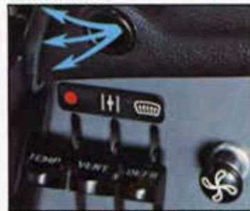
Ventilation and heating control levers.
