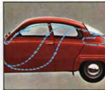
Air circulated through car and out rear.
