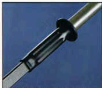
Collapsible steering column.
