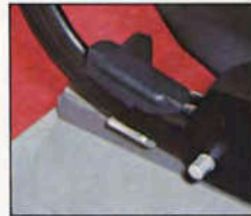
Catch to prevent seat from tipping forward.
