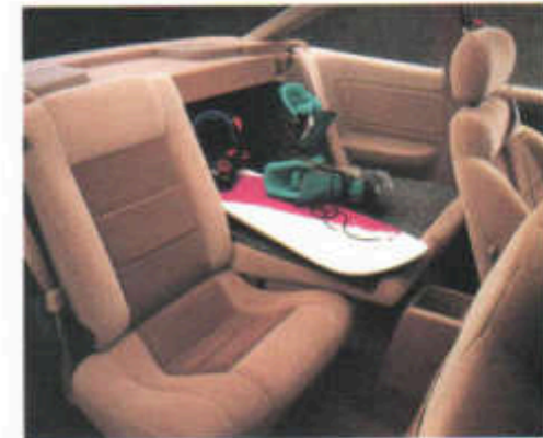
In all three Saturn sedans and in the coupe (featured above), the rear seatback splits and folds down to make toting big, cumbersome things that much easier. In fact, the sedans come with three safety belts in the rear seating area, so that you can fit two small children in the larger seat, and fold down the smaller seat for packages.
