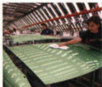
Dent-resistant polymer body-side panels are among the design team's more intriguing innovations. The panels are painted with a primer coat that flexes on impact, a waterborne acrylic color basecoat that looks wet and low-trim, and a clearcoat tough enough to fend off tree sap, ultraviolet light, and even the most wayward pigeon. Recyclable and resilient, they won't rust, oxidize, or fall prey to the usual nicks, dents, or dings inflicted by such everyday hazards as shopping carts, car doors, or even young Monica, the budding neighborhood T-ball champion.
