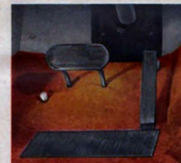
No clutch pedal on Automatic Drive models. The brake pedal is oversize—may be used with either foot. For your added safety, engine won't start unless selector is at "N" or "P."
