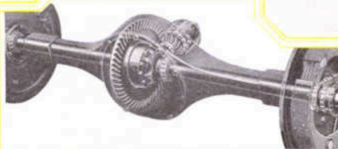
A "phantom" view of the special heavy duty rear axle—note the heavy box section housing and large shafts.
