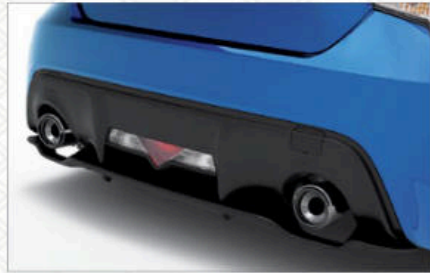
Rear Diffuser. Lower rear body panel helps to direct airflow and adds a sculpted finishing touch to the BRZ lower rear body line.
