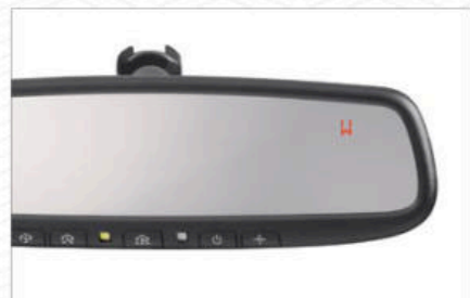
Auto-dimming Mirror with Compass and HomeLink®. Mirror darkens when headlights are detected from behind the vehicle. Includes a compass and three HomeLink® buttons that are programmable for most garage-door openers and other HomeLink®-compatible devices.
