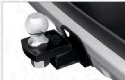
Trailer Hitch. Subaru hitches are engineered to the same rigorous standards as the rest of the Outback. Heavy-duty rated at 3,500-lb. towing capacity, 350-lb. tongue weight, for the 2.4L Turbo XT and at 2,700-lb. towing capacity, 270-lb. tongue weight, for the naturally aspirated 2.5L.
