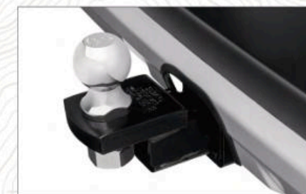
Trailer Hitch. Subaru hitches are engineered to the same rigorous standards as the rest of the Outback. Heavy-duty rated at 3,500-lb. towing capacity, 350-lb. tongue weight, for the 2.4L Turbo XT and at 2,700-lb. towing capacity, 270-lb. tongue weight, for the naturally aspirated 2.5L. Hitch ball not included. Ball mount sold separately. Trailer brakes may be needed.
