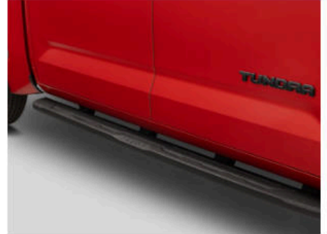
TRD cast-aluminum running boards
