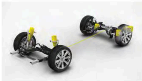
Air suspension on all four wheels gives the XC90 outstanding ride comfort – the air springs absorb imperfections in the road – and make the car stable by keeping the ride height constant, regardless of the load. With the active chassis you can alter the way the car rides and handles to suit your mood or the road.
